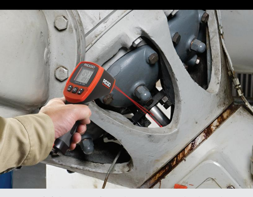
The RIDGID® micro IR-200 Non-Contact Infrared Thermometer provides simple, quick and accurate surface temperature readings at the push of a button. Simply squeeze the trigger and point the ultra-sharp dual class II lasers at the surface being measured.
